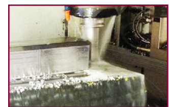
Inconel machining with the new SPINWORX® DR12-8B3 insert
